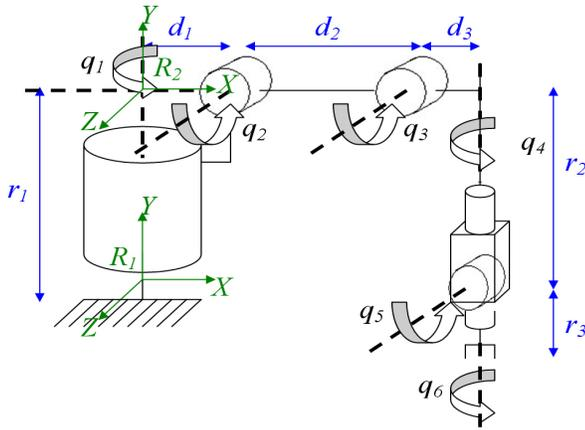
Figure 2. Parameters used for the direct geometrical model of the Kuka Kr6.
