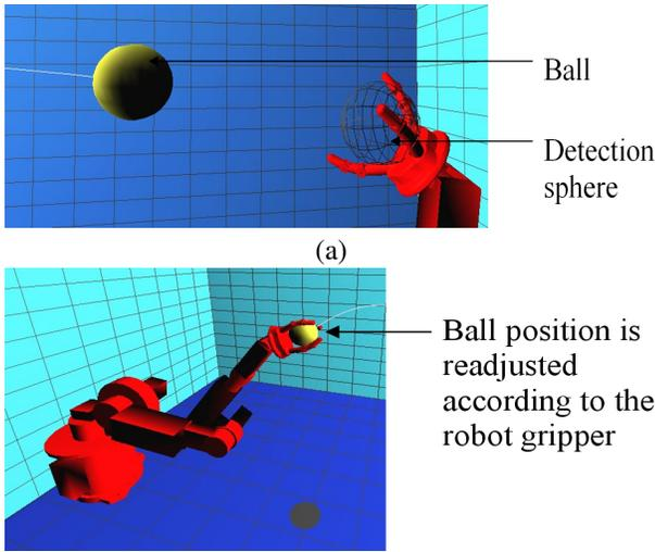
Figure 3. Grasping system: (a) the detection sphere and the flying object. (b) the ball centre is inside the detection sphere, so the dynamic object position is readjusted to the gripper position.
