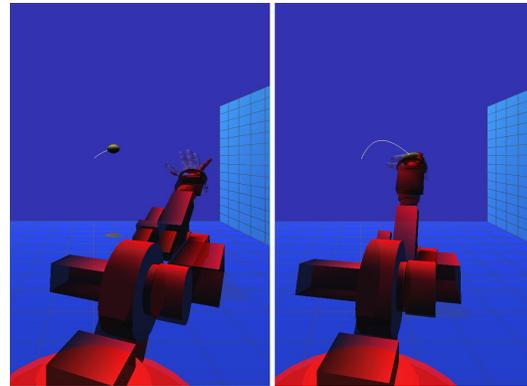
Figure 5. The user vision during the learning process. The robot is driven by user to grasp the flying ball.
