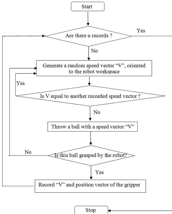
Figure 6. Diagram of the demonstration process (n: number of required demonstrations).
