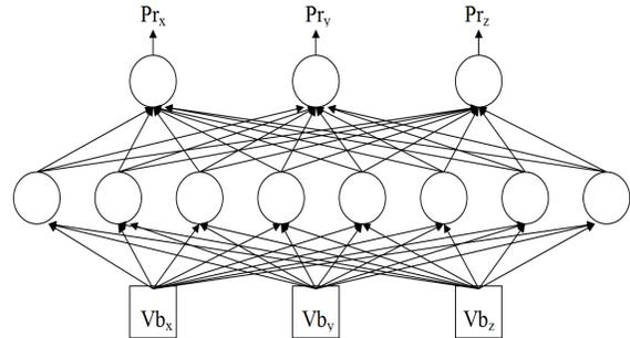
Figure 7. Neural network used for this experiment: 3 inputs, 8 neurons in 1 hidden layer, 3 output neurons, activation function: sigmoid exponential function and  $n = 0.2$  ( $n$ : learning rate).
